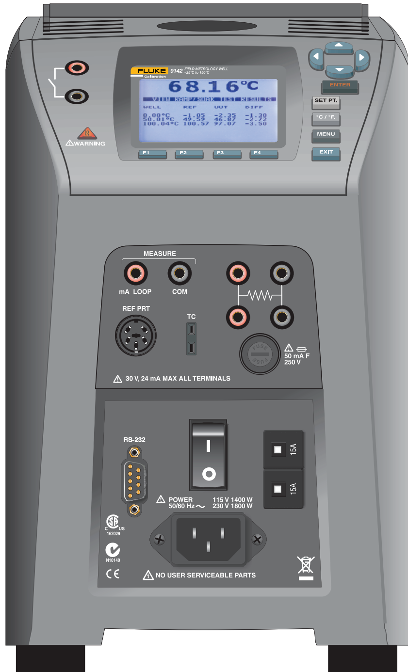
Рис. 2. 914X Field Metrology Well
